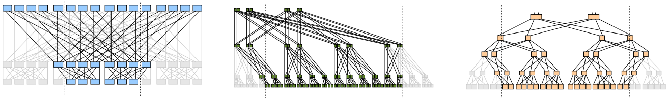
Fig. 3. "Partial" construction of the topologies: 4,3-fat-tree (left), 4,2,4-thin-tree (middle) and 4,2,5-slender-tree (right).
