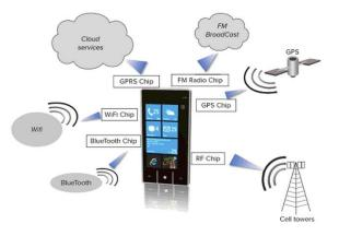
Figure 5 shows smartphone device wireless network interfaces.
