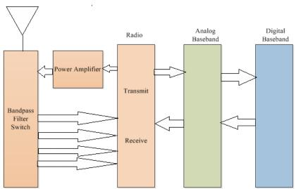
Two Sections Circuts of A Radio Transciever
