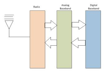
Figure 1.Block Diagram of GSM Modem components
