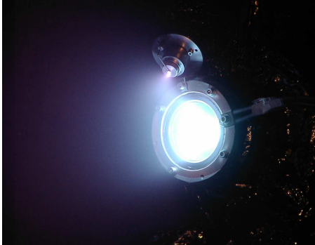
Figure 6: HKN 5000 BB-3 mounted on HEMP-T 3050 DM8 in operation during a 250h endurance test
