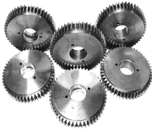
Fig. 4 The test gear pairs used in this study: (a) \delta=0 , ICR =1.8; (b) \delta=10 \mu\text{m} , \alpha=20.9 \text{ deg} , ICR=1.8; and (c) \delta=0 , ICR =1.4
