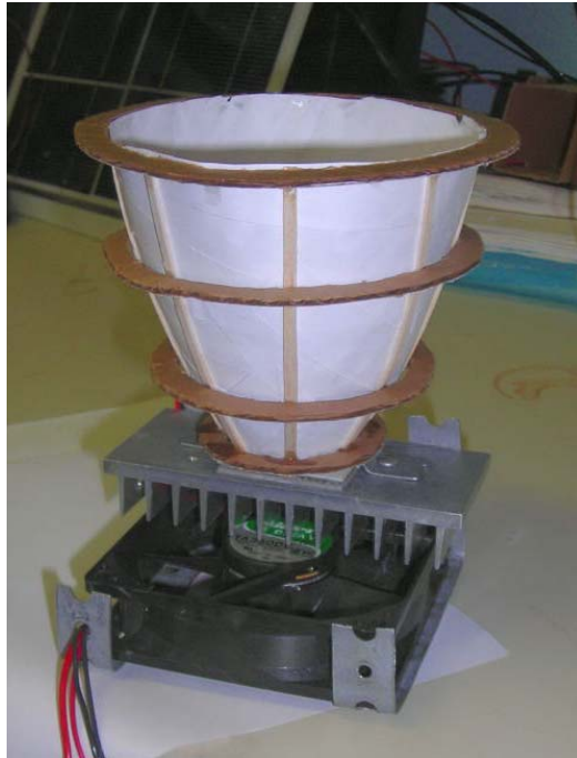
FIG.5. THE EXPERIMENTAL CPC/TEM THERMOELECTRIC GENERATOR SETUP.
