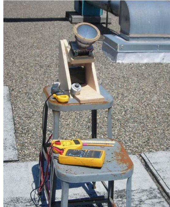
FIG. 6. THE EXPERIMENTAL SETUP MOUNTED ON A MANUAL SOLAR TRACKER AND PLACED IN THE SUN.
