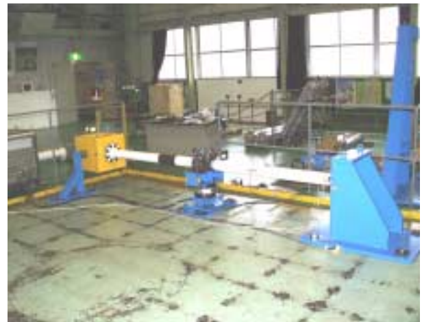
Fig.3 Photograph of U-bolt element test model
