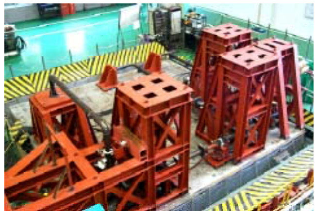
Fig. 10 Photograph of full-scale piping model excitation test
