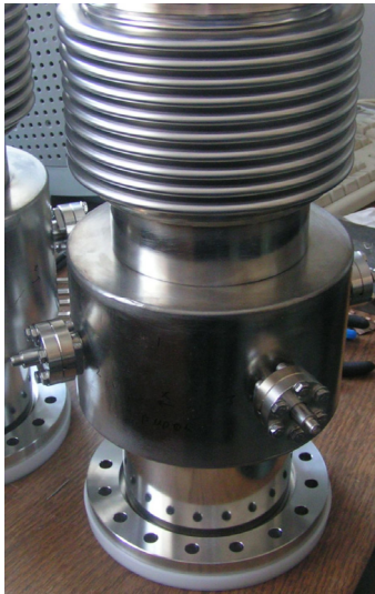
Fig.2. A piece of vacuum chamber with BPM.
