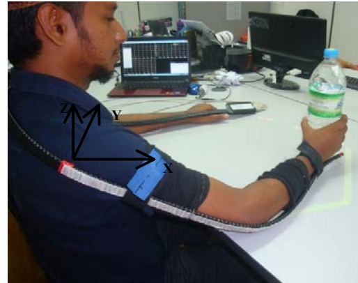
Figure 2. Shapetape® mounted on subject's arm
