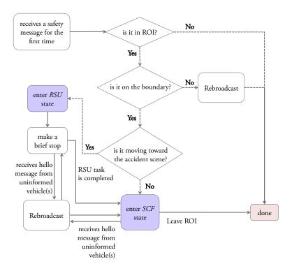
Fig. 2. Flow diagram describing the distributed algorithm for selecting a temporary RSUs and the tasks performed by temporary RSUs.
