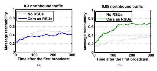
Fig. 5. Impact of the mobility pattern on the message reachability of the network with and without RSU-vehicles. The improvement of RSU-vehicle scheme over the conventional scheme increases with the increase in northbound traffic. The results are based on a 1 km x 1 km Region of Interest network with vehicle density of 100 veh/km<sup>2</sup>, 20% DSRC penetration rate, and 30-second RSU-vehicle stop time.
