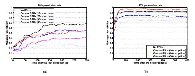
Fig. 4. Impact of the RSU-vehicle stop time on the message reachability of the network with and without RSU-vehicles. Substantial improvement is observed only in sparse and moderately-dense network. The results are based on a 1 km x 1 km Region of Interest and vehicle densities of 100 veh/km<sup>2</sup> with 20% and 40% DSRC penetration rates on the left and right figures, respectively.
