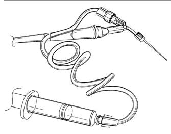
Figure 2. Diagrammatic representation of ultrasonic irrigating device used in this study.
