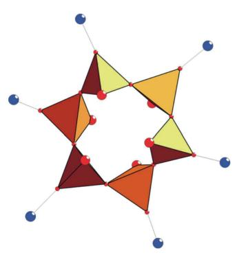
Fig. 1. Lovozerite-type ring  $[Si_6O_{12}(O,OH)_6]$ ; small circles are O atoms forming the bridges Si–O–Si and Si–O–M, large circles in "pendent" vertices of Si tetrahedra represent (O,OH), large circles connected with small circles are M cations.
