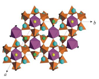
Fig. 2. Structure of lovozerite (after Yamnova *et al.*, 2001a): Si tetrahedra, M octahedra, C (small circles), A (medium circles) and B (large circles) sites are shown.
