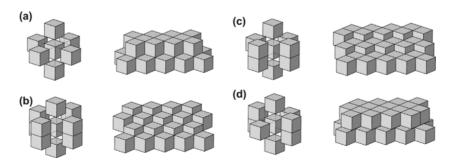
Fig. 4. Four types of arrangements of cubic modules in the lovozerite structure-types: (a) in trigonal members; (b) in imandrite; (c) in koashvite; (d) in synthetic  $Na_5(Na_{0.5-x}/2(Nd_xCa_{1-x})_2(Si_6O_{18})$ .
