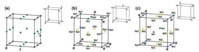
Fig. 6. Location of the A, B, and M cations relative to the outline of the cubic module in minerals of the lovozerite group: (a) the lovozerite-zirsinalite subgroup, (b) the koashvite subgroup and (c) the imandrite subgroup. The insets show the location of the M-type cations.
