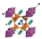
Fig. 3. Pseudocubic ( $a' \approx 7.5$  Å) module in the lovozerite structure-type. The arrow along the space diagonal in the cube represents a three-fold axis. A sites are on the cube edges, B sites centre the cube faces and C sites are on the three-fold axes.
