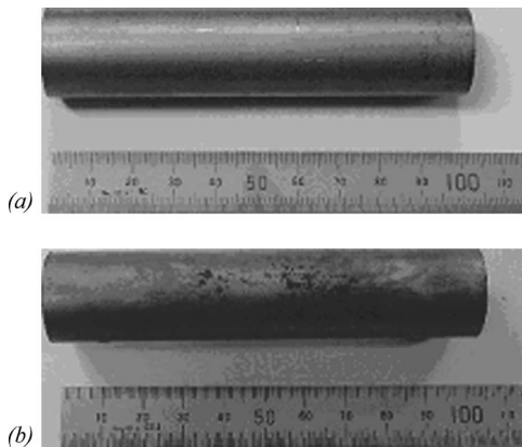
Fig. 3 Photographs of SUS 304 pipe before and after the application of shock wave at cryogenic temperature (87 K). (a) Before; (b) after.
