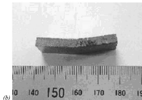
Fig. 5 Photograph of shocked SUS 304 at cryogenic temperature (87 K). (a) Top view; (b) side view.
