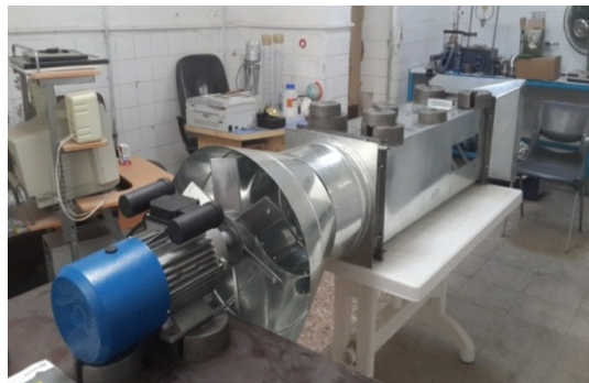
Figure-2. Different parts of the manufactured wind tunnel
