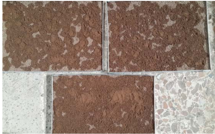
Figure-6. Changes on soil surface due to different heights for solutions fall
