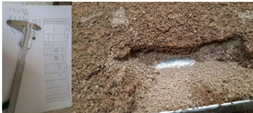
Figure-7. Cut soil section for solutions penetration depth measurement
