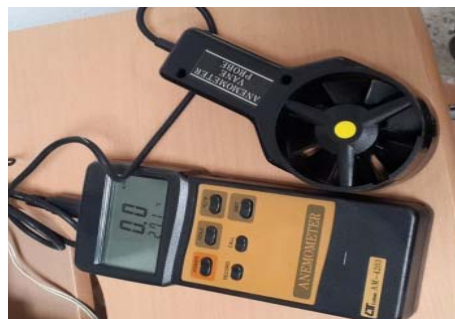
Figure-3. Handheld anemometer used for test
