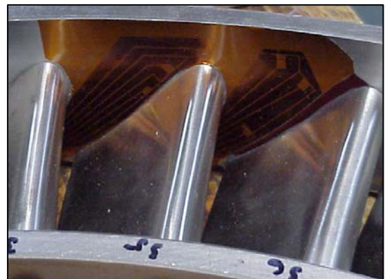
Figure 3. Photograph of the turbine vane OD endwall instrumented with thin film heat flux gauges.
