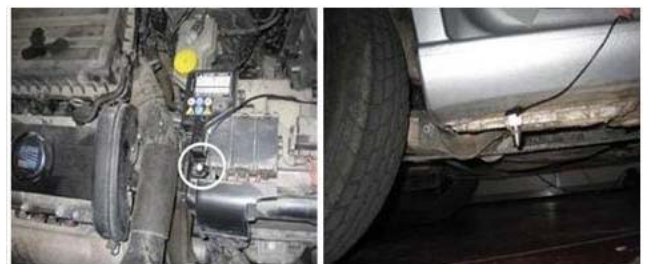
Figure 4: Microphones installed in engine compartment and vehicle chassis underbody
