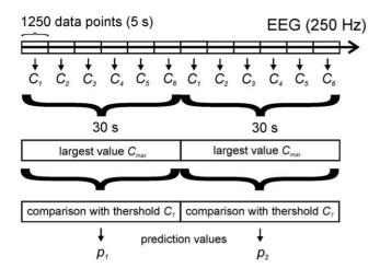
**Figure 1. Principle of analysis.** 5 s long successive data segments are analyzed by RQA yielding complexity values  $C_1...C_n$ . From 6 consecutive  $C_i$ 's, the largest values  $C_{max}$  are compared with a threshold  $C_T$  to generate the decision values  $p_i$  for making a conscious/ unconscious decision.
