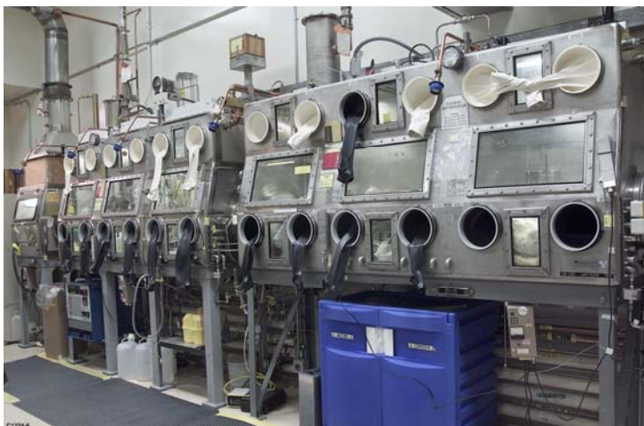
Figure 1. Typical Glovebox Train.
