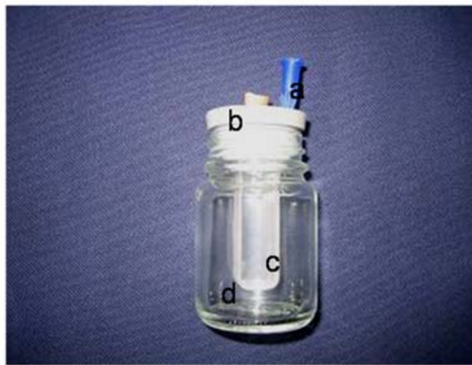
Fig. 1: Assembly prepared to collect the apical debris during removal of RealSeal™
