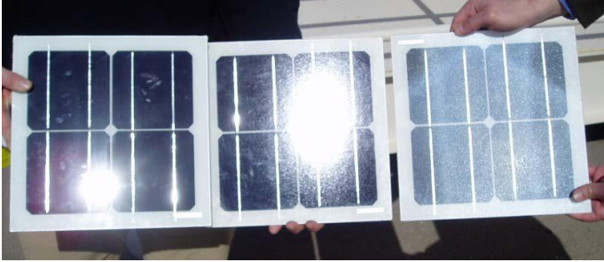
Figure 2. Examples of solar glare and beam spread resulting from different PV glass samples, with varying surface texture, captured with a digital camera (Permission from [3]). Left: smooth glass. Middle: Lightly textured glass with anti-reflective coating. Right: Deeply textured glass. Samples courtesy of Canadian Solar, Inc.
