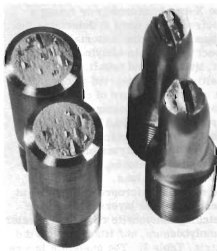
Fig. 2—Fracture appearance of smooth and notched tension-test specimens of maraging (250) steel showing longitudinal "splits" and "internal shear lips".
