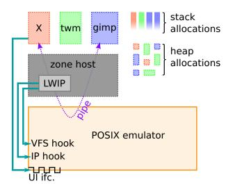
Figure 2: Multiple POSIX apps coexist in one picoprocess as zones. Each zone comprises a noncontiguous partition of the address space. Each has its own copies of libraries, like libc, and its own stack and heap allocations. Programs that expect POSIX pipe IPC, such as an X session, see the same behavior within the picoprocess.
