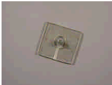
Figure 5 Photograph of the bonded part for PDMS diaphragm, PMMA layer and bulk magnet.
