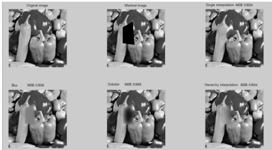
Figure 4.1 (a): Original image (b): image with mask values zero (c):image inpainted by interpolation (d): image inpainted by blur (e): image inpainted by Sobolev method (f): image inpainted by Hierarchical method
