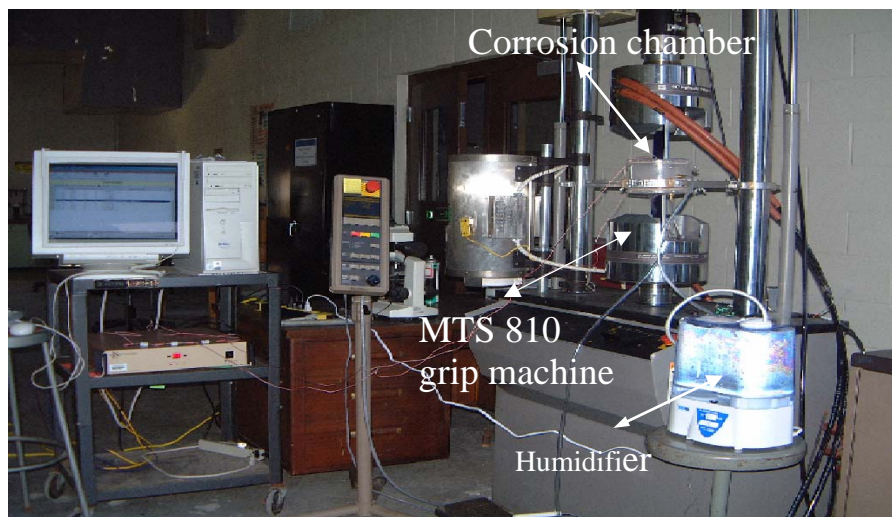
Figure 2.2 Experimental facilities (MTS-810, Strain smart software, and Corrosion chamber)
