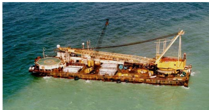
Figure 1: The BGL-1 Pipeline Launching Barge
