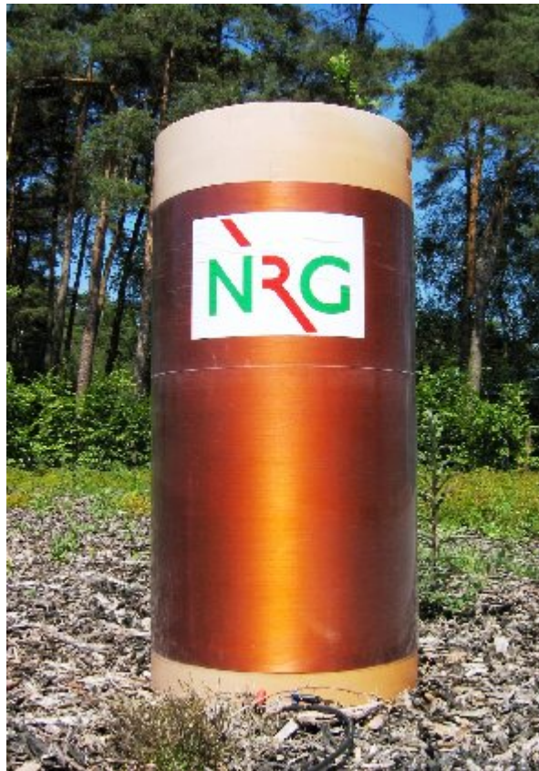
Fig. 2. Receiving antenna NRG-4.
