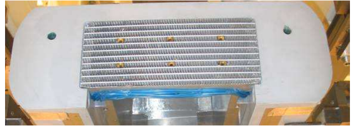
Figure 12. Radiator core equipped with 6 Probes
