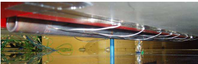
Figure 3. Heated plug in the underbody evacuation duct
