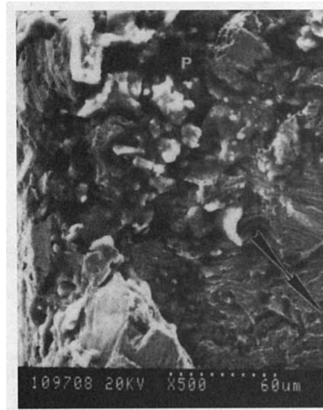
Fig. 7 A crack initiation site near the surface of the weld toe, for specimen 3. The arrow indicates the direction of crack growth.
