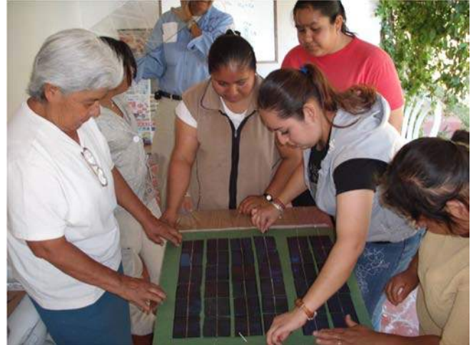
Fig 11 Women in Mexico learning how to build a 30 watt PV module at the Villa Energia cooperative they started.
