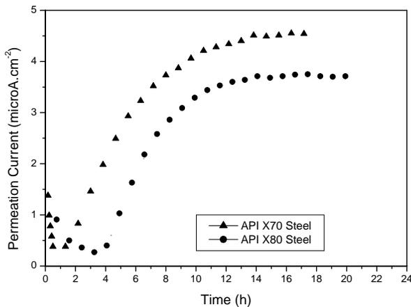
Figure 1 – Hydrogen permeation current obtained for API-X70 and API-X80steels in sodium thiosulphate solution.
