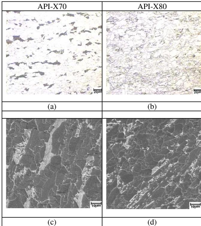
Figure 2 – Optical Micrographs (a,b) and Scanning Electron Micrographs (c, d)
