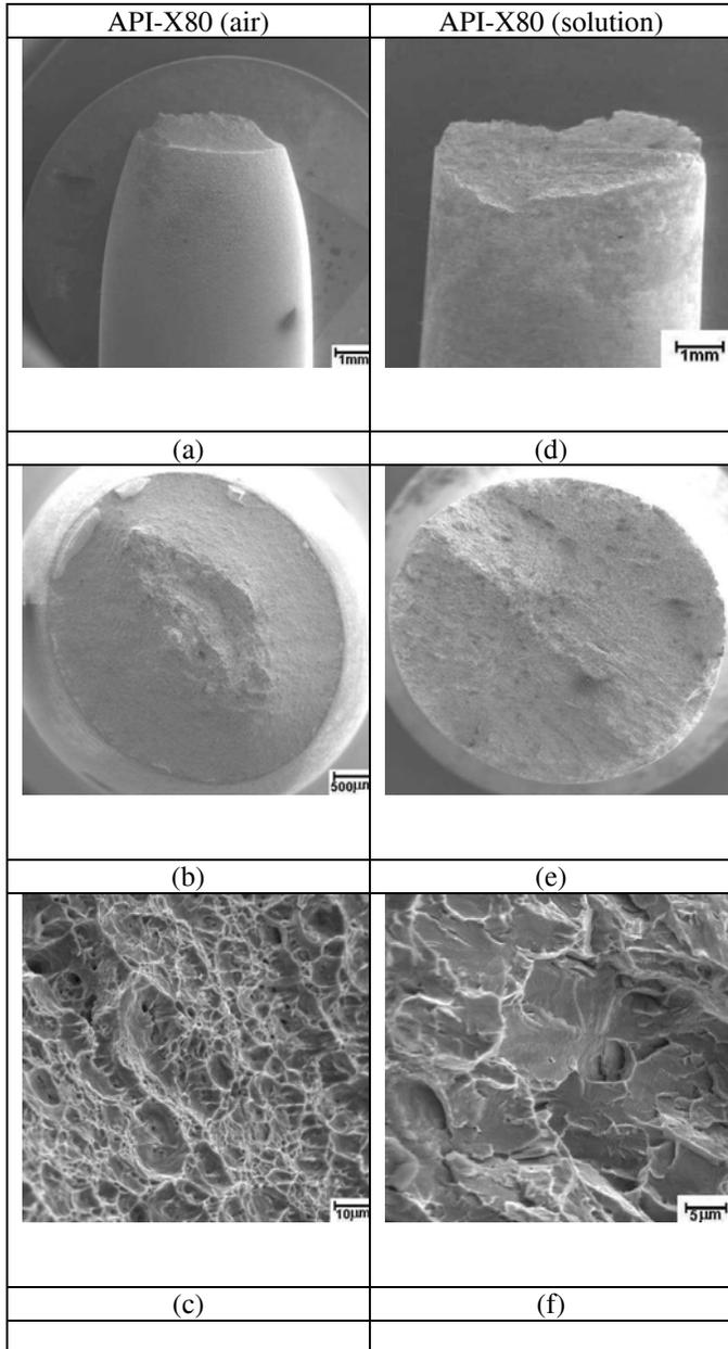
Figure 3 –SEM analysis of API-X80 testpieces tested in air (a,b,c) and in the Thiosulphate-based Solution (d,e,f)
