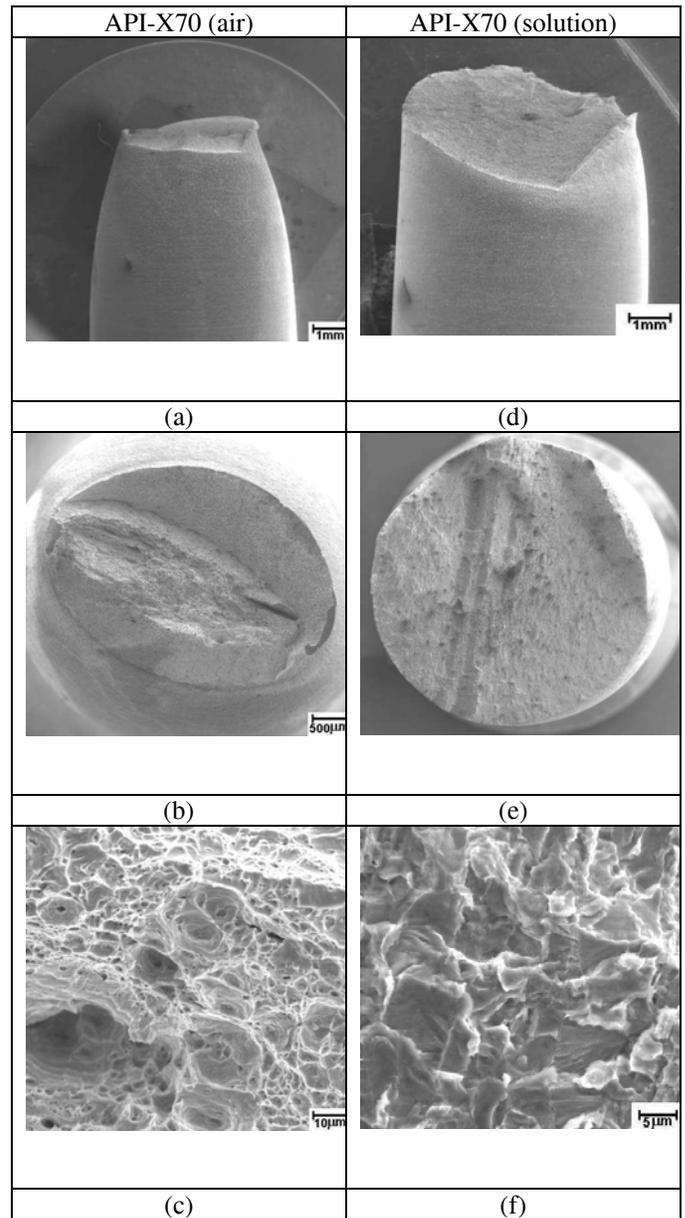
Figure 2 –SEM analysis of API-X70 testpieces tested in air (a, b, c) and in the Thiosulphate-based Solution (d, e, f)
