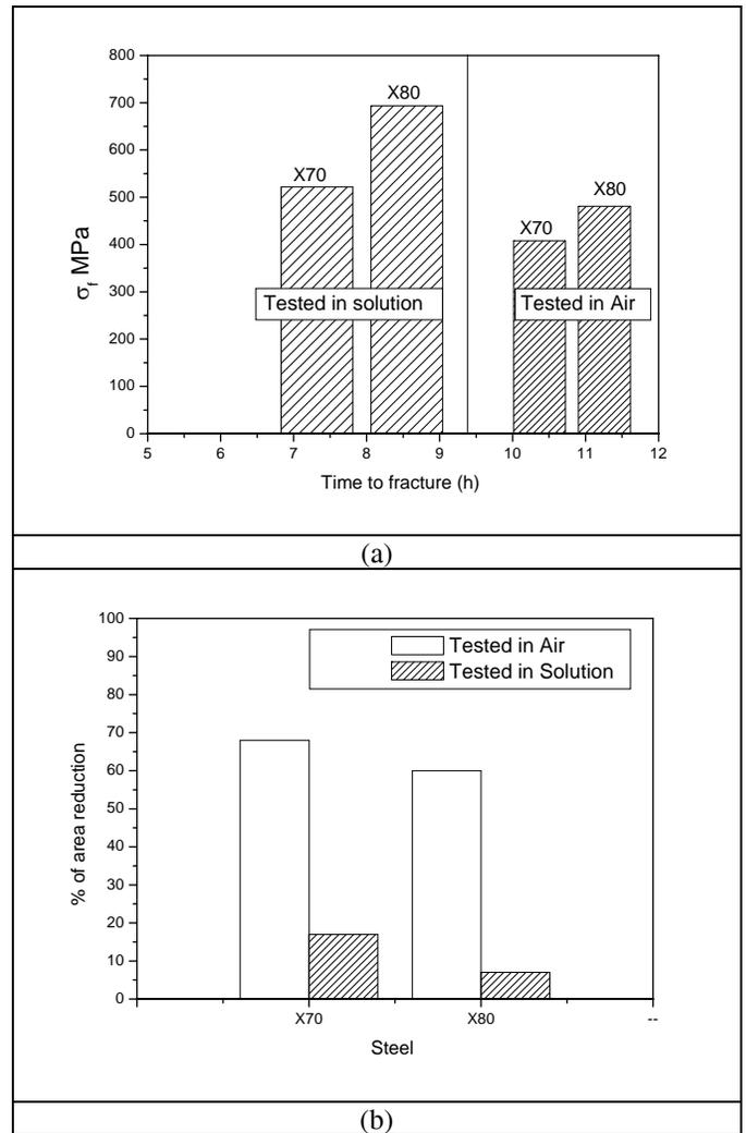
Figure 4- Behaviour of API-X70 and API-X80 when tested in air and in thiosulphate solution, (a) time to fracture and (b) % of area reduction.
