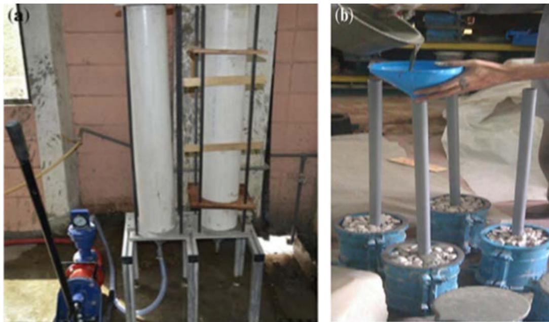
Fig. 1 Methods of grouting in two-stage concrete: (a) pump method and (b) gravity method
