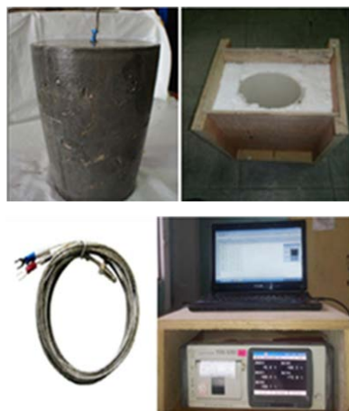
Fig. 3 Test setup for the measurement of heat of hydration
