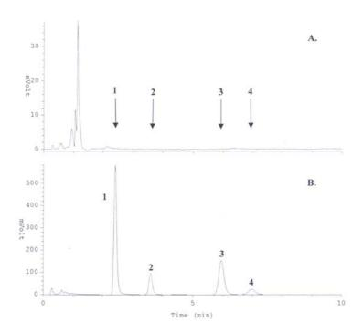
**Fig. 1**Chromatograms obtained from vehicle gel extract (A) and Flucinar gel extract (B) containing of nipagin M (1), nipagin A (2; internal standard), nipagin P (3) and fluocinolone acetonide (4) at concentrations 155, 30, 86, and 23.25 μg mL<sup>-1</sup>, respectively
