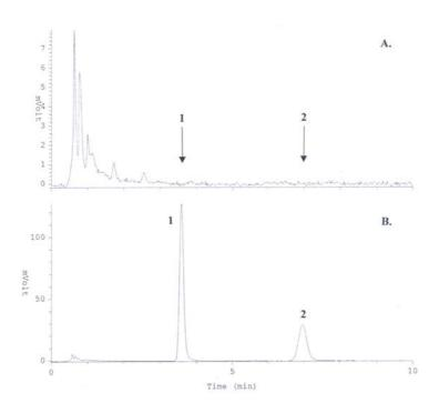
**Fig. 2** Chromatograms obtained from vehicle ointment extract (A) and Flucinar ointment extract (B) containing 22.75  $\mu$ g mL<sup>-1</sup> fluocinolone acetonide (1) and 30  $\mu$ g mL<sup>-1</sup> nipagin A (2; internal standard).
