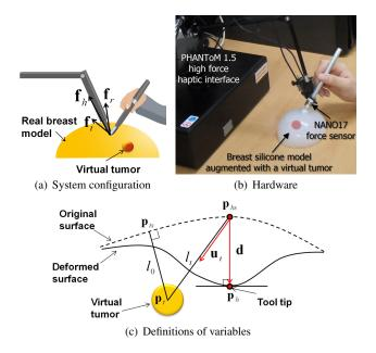
Figure 1: System configuration and variables definition.
