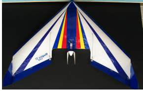
Fig. 2. An in-house fixed-wing semi-autonomous mini-UAV
