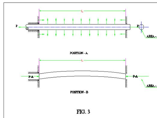
$$M = \int_x^l A \left( \frac{dp}{dx} \right) (\eta - y) d\xi \quad . \quad . \quad (3)$$
