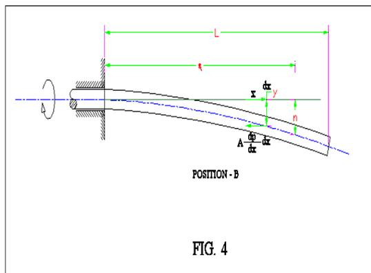
Where  $y$  is the deflection at section  $x$  and  $\eta$  is the deflection at section  $\xi$ , and this may cause buckling if it exceeds the elastic restoring moment in the shaft. It will be clear from this discussion that the body forces
