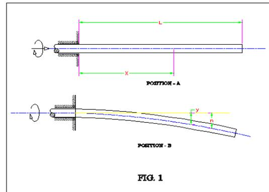
**BUCKLING OF A NON ROTATING SHAFT**
