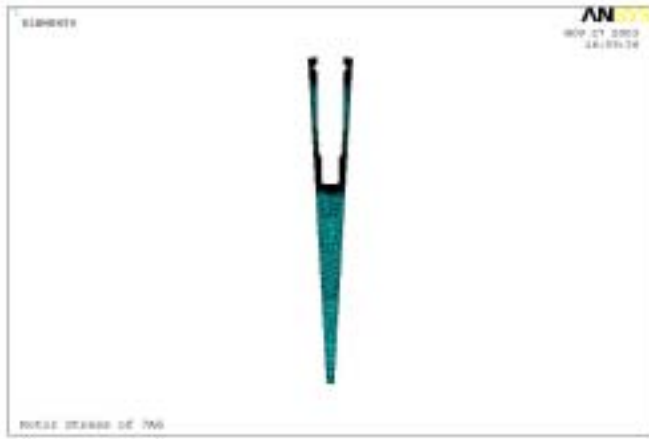
Figure 4: FEM model of rotor tooth.
