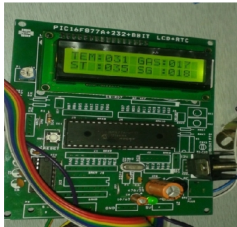
Figure.7 Temperature and Odour Senssing
