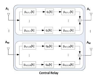
Fig. 2. Block diagram of the central relay with pre/post-rake filtering and equalization filtering for multiuser two-way FF relaying.
