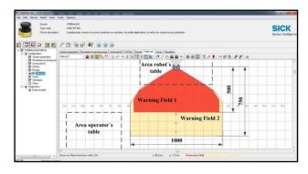
Figure 3. Drawing of the proposed 2D laser scanner security zones
