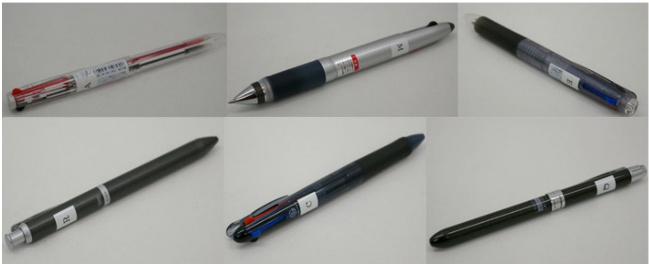
Figure 1. Pens A-M-E (upper row) and R-C-Q (bottom row). Pen A has a transparent plastic cover, pen C and E have semitransparent plastic cover. Pen R has a metallic cover with a matte finish. Pen Q has a metallic cover with a glossy finish.
