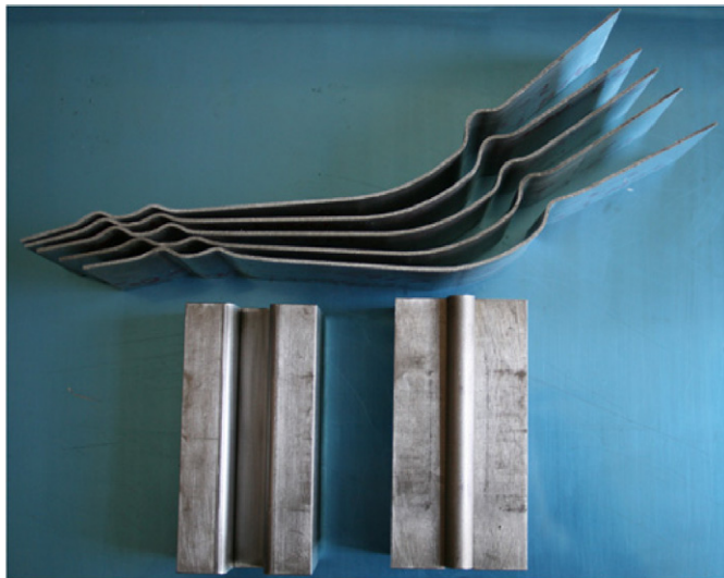
Fig. 7. Experiment results and inserts of draw-bead test device.
