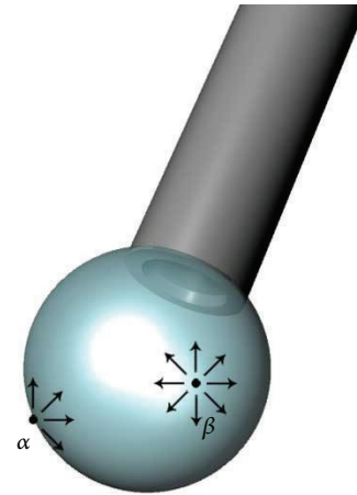
FIGURE 1: Droplet of water at the end of a pipette. Molecule \beta , which is positioned inside the droplet, is equally attracted in all directions. Molecule \alpha , which is located on the surface, is exposed to more attractive forces inside rather than outside the droplet, and the resultant attractive force is thus inwards. Surface tension acts like a film as it tries to achieve the smallest surface area for a given volume (modified from Kirchhof and Wong [74]).
