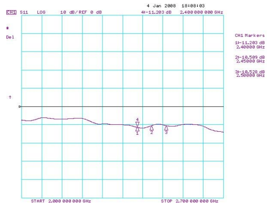
Fig. 7 LOG MAG value is about -10dB with short-type transmission line under 2.4~2.5GHz operation.
