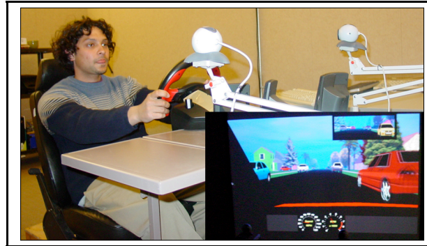
Fig. 1. Participant being monitored in STISIM driving simulator
