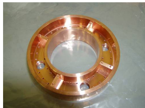
Figure 3. A segmented plenum chamber
