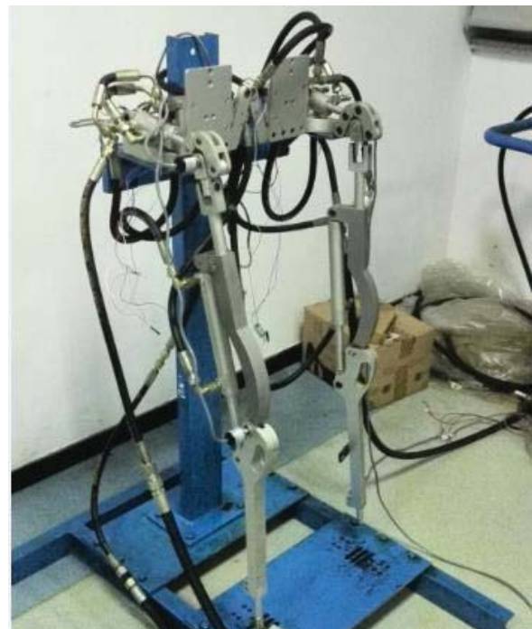
FIGURE 1. An exoskeleton system with electro-hydraulic actuation.
