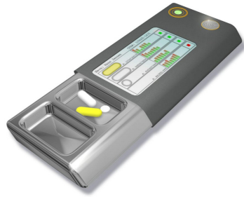
Figure 3: The Context-Aware Pill Container. a – the vision with fingerprint recognition and a LED indicating proximity to the patient. b – the current prototype based on RFID technology.
