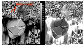
Figure 3 (left) Nano-porosity Available in the Calcium Silicate Grain Fabric Shown in a BSE image Plug #24. (Right) Plug #24 Elemental Calcium-Silicate Mapping Shows Maps of Calcium And Silicon.
