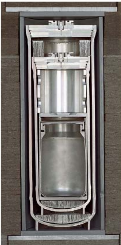
Figure 2 – 9975 Cutaway View with 3013
