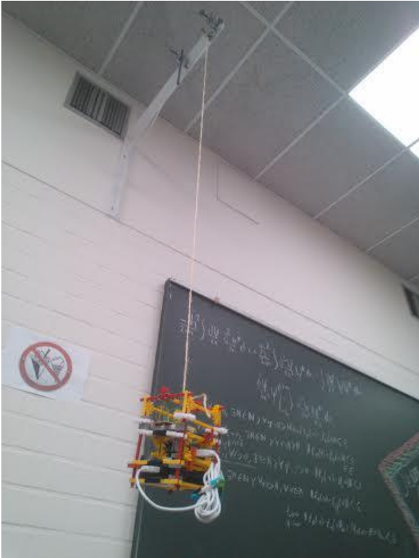
Figure 6. Experimental setup to test the 3-axis accelerometer
